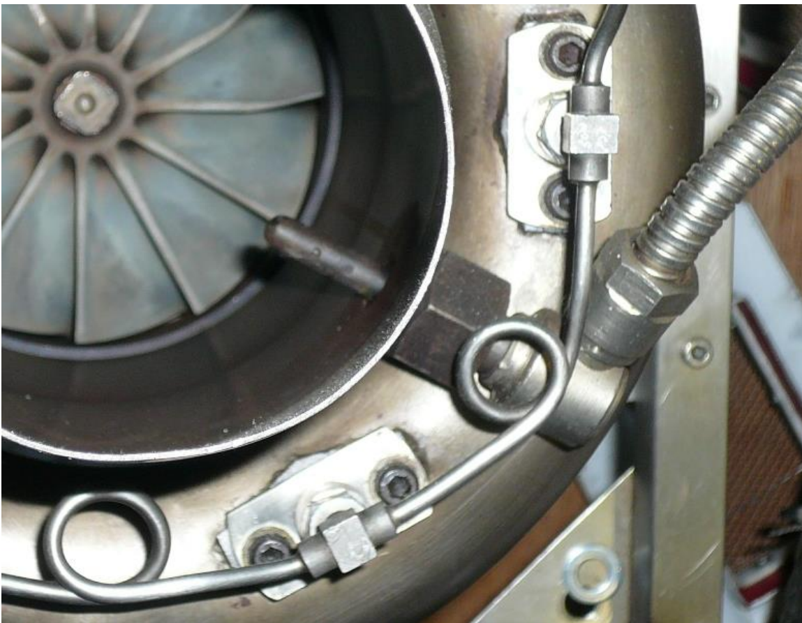
Single engine mounted EGT thermocouple stagnation-type probe.
