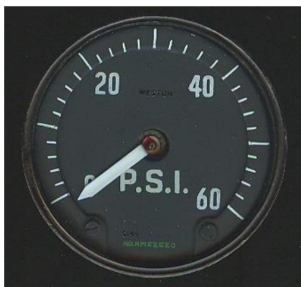
Weston "ratiometer" oil pressure indicator
