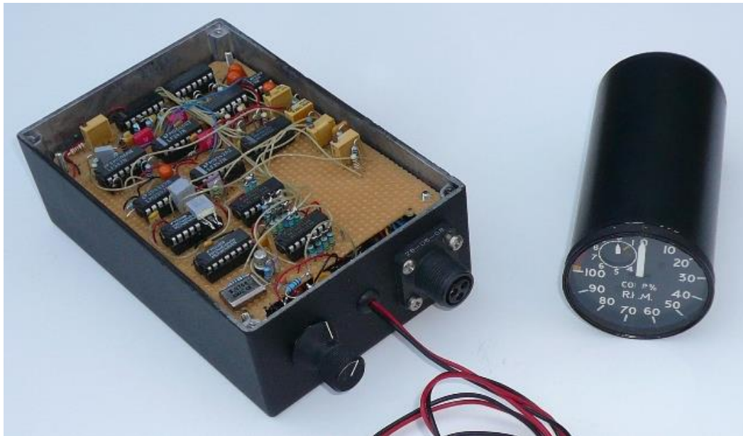
Electronic 3-phase test generator for operating percent indicators
