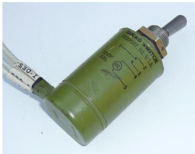
Picture switch with hold-in coil
