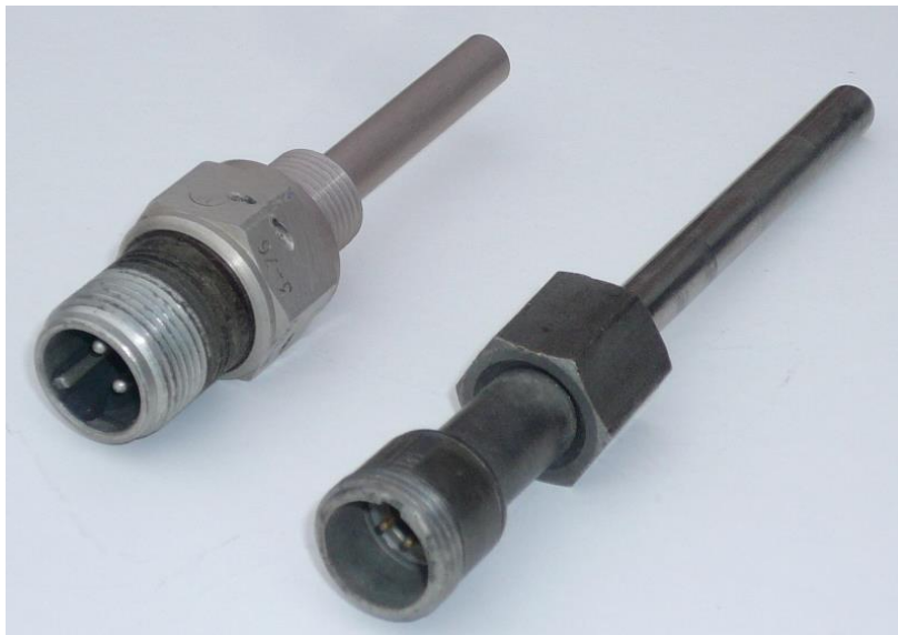
Thermistor oil temperature sensor probes
