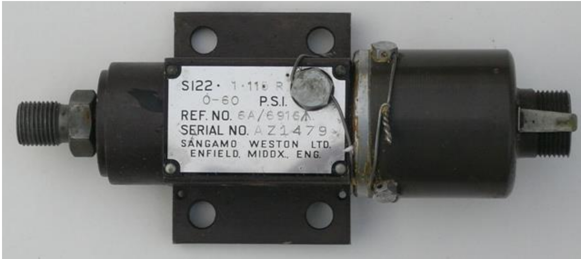
Weston oil pressure DC ratiometer type sender unit
