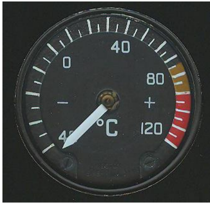
Weston "Ratiometer" oil temperature indicator
